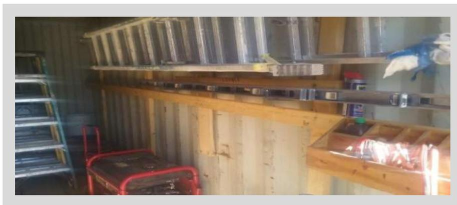
The Level Holder shown on the drawing is only needed on one rack per container and can be built by using a piece of 2x4 long enough to span between the legs of the Rack, and two ladder hooks. Space the hooks no more than 3' apart and the rack can hold all three sizes of levels.
